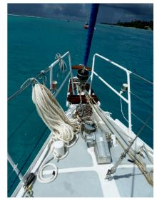
**Midships:** 10mm baby stay, two lower, two mid and two higher shrouds and the running backstays are to be found here. The guardrail can be opened on both sides using pelican hooks. Two solid cleats are mounted on both sides. Two dorade vents direct fresh air into the saloon.
