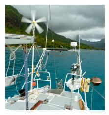
**Bathing platform:** Made from stainless steel/teak, permanently mounted with folding stainless steel ladder. Rock solid 'Fleming' wind vane mounted to the stern. Underneath is a drum with 200m of floating line for the horseshoe buoy. Standing on the starboard side: a 35kg anchor.
